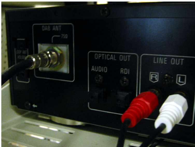
Figure G.17: Rear of DAB tuner
