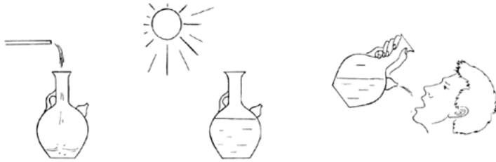
Figure 1.11: Solar disinfection of drinking water. The illustration shows water in a common drinking jug of glass being exposed to the sun. (From [5])
