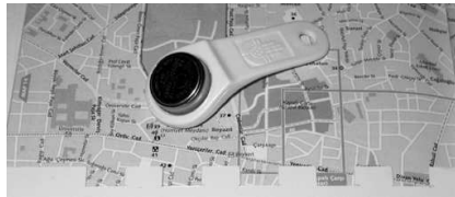
Figure 1.15: The Akbil iButton digital ticket holder is about the size of an ordinary latch key.
