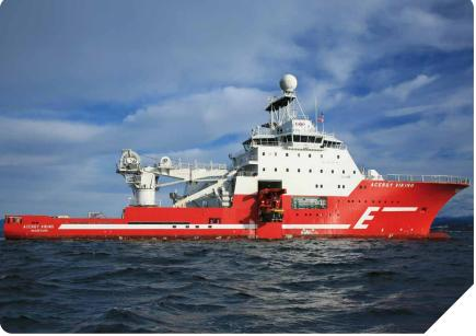
The Acergy Viking is a new generation IMR, Survey and Light Construction vessel, with a fast transit speed and is ideally suited for operations in harsh environments.
